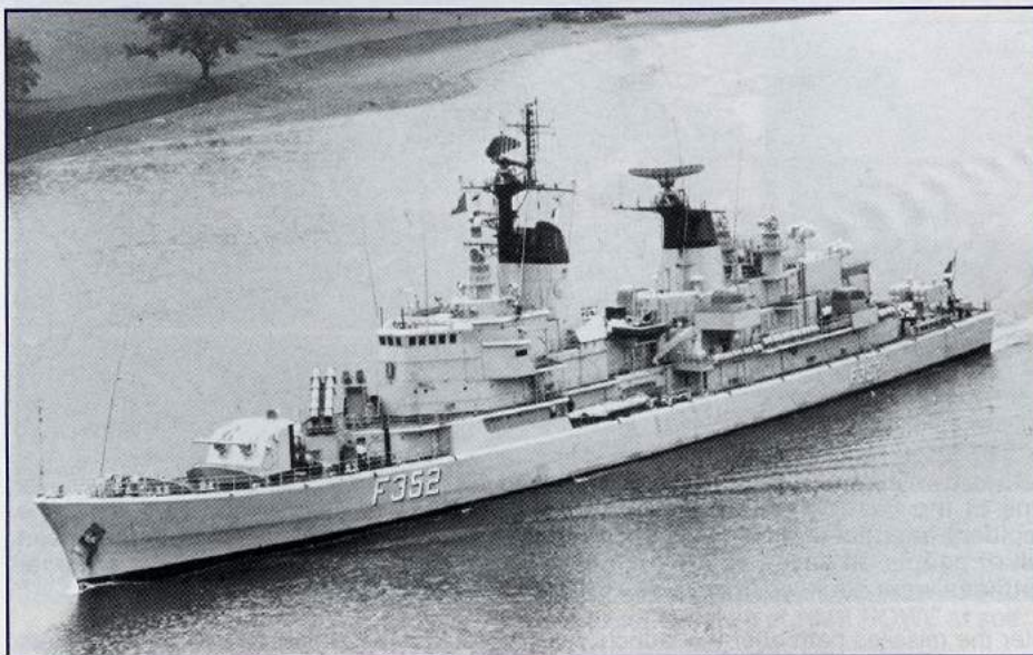
The frigate PEDER SKRAM. Launched in 1965 as a part of the Danish-American arms agreement of May 1959. The ship was originally armed with 2 x 2 5-inch guns, but one of the two turrets was removed in 1977-79 and replaced with eight Harpoon-missiles. It had a crew of 178, a maximum speed of 30 knots and a displacement of 2400 tons.
